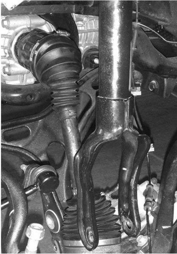
Remove the bolt from the forward end of the lower control arm.
